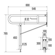
Bright polished 304 stainless steel tube Ø 32 mm. Bright polished stainless steel flange. Bright polished 304 stainless steel support prop adjustable, Ø 25 m, for hinged bar. Visible fixings.
