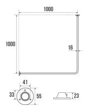
Chrome and nickel-plated steel tube Ø 16 x 0,5 mm. Can be cut to size. 2 sliding wall flanges made of white ABS.
