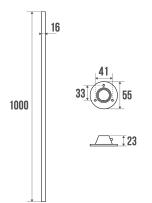
Chrome and nickel-plated steel tube. Can be cut to size. 2 sliding wall flanges made of white ABS.
