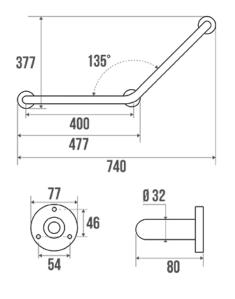
3 fixing points. 400 x 400 mm symmetric grab bar. Bright polished 304 stainless steel tube Ø 32 mm. Bright polished stainless steel cover plates and flanges. Wall fixings included. Incompatible in chlorinated environment.
