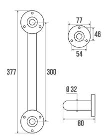
Bright polished 304 stainless steel tube Ø 32 mm. Bright polished stainless steel cover plates and flanges. Wall fixings included. Incompatible in chlorinated environment.
