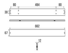
Fixing rail fitted with an anodised aluminium cover, with 2 anthracite resin bolts. The cover can be replaced by a straight grab bar 662 mm or a backrest + 2 armrests or a backrest + 2 hinges bars for shower seat and can thus be used to convert a "Classic" shower into an accessible "Comfort" shower.
