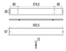
Fixing rail fitted with an anodised aluminium cover, with 2 anthracite resin bolts. The cover can be replaced with a straight grab bar 552 mm or a backrest + 1 armrest or a backrest + 1 hinged bar for shower seat and can thus be used to convert a "Classic" shower into an ergonomical "Comfort" shower.
