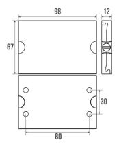
Fixing rail fitted with an anodised aluminium cover, with 2 anthracite resin bolts. The cover can be replaced with a hinged grab bar or an armrest and can thus be used to convert a "Classic" shower into a "Secure" shower.
