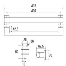
Elliptical tube in bright chrome-plated aluminium  $38 \times 25$  mm. Chrome-plated resin flanges.
