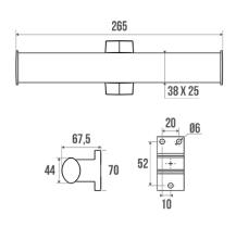
Elliptical tube in bright anodized aluminium 38 x 25 mm. Chrome-plated resin flanges.
