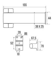
Elliptical tube in bright anodized aluminium 38 x 25 mm. Chrome-plated resin flanges.
