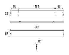
Fixing rail fitted with an anodised aluminium cover, with 2 white resin bolts. The cover can be replaced by a straight grab bar 662 mm or a backrest + 2 armrests or a backrest + 2 hinges bars for shower seat and can thus be used to convert a "Classic" shower into an accessible "Comfort" shower.
