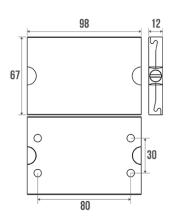
Fixing rail fitted with an anodised aluminium cover, with 2 white resin bolts. The cover can be replaced with a hinged grab bar or an armrest and can thus be used to convert a "Classic" shower into a "Secure" shower.
