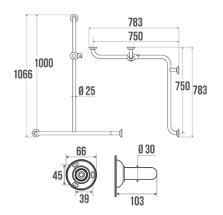
White epoxy-coated aluminium tube Ø 30 mm. 90° angled. White epoxy-coated resin flanges and cover plates.
