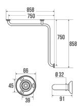
Chrome and nickel-plated brass tube Ø 32 mm. 90° angled. Bright chrome-plated resin flanges and cover plates.
