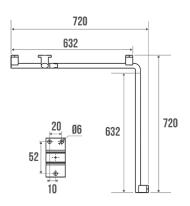
Elliptical tube in white epoxy-coated aluminium, 38 x 25 mm.
