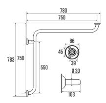
White epoxy-coated aluminium tube Ø 30 mm. 90° angled. White epoxy-coated resin flanges and cover plates. 3 concealed fixing points. Screws included.
