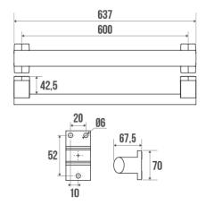
Elliptical tube in anthracite grey epoxy-coated aluminium, 38 x 25 mm. Anthracite grey epoxy-coated resin flanges and cover plates. Screws included.
