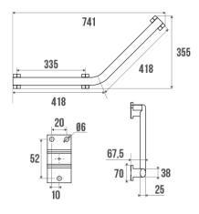
3 fixing points. 400 x 400 mm symmetric grab bar. Elliptical tube in anthracite grey epoxy-coated aluminium, 38 x 25 mm. Anthracite grey epoxy-coated resin flanges and cover plates. 3rd point to be fitted for right or left version. Screws included. Anticorrosion warranty. Design coordinated with all ARSIS Comfort items.
