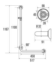
Chrome and nickel-plated brass tube Ø 32 mm. Bright chrome-plated resin flanges and cover plates.
