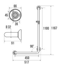
Chrome and nickel-plated brass tube Ø 32 mm. Bright chrome-plated resin flanges and
