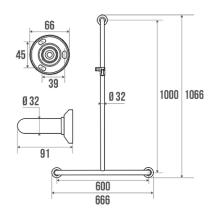
Chrome and nickel-plated brass tube Ø 32 mm. Bright chrome-plated resin flanges and cover plates. With slider bracket for shower handset in metallized finish ABS.
