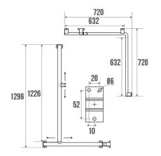
Elliptical tube in white epoxy-coated aluminium, 38 x 25 mm.
