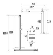
Elliptical tube in white epoxy-coated aluminium,  $38 \times 25$  mm. White resin cover plates.
